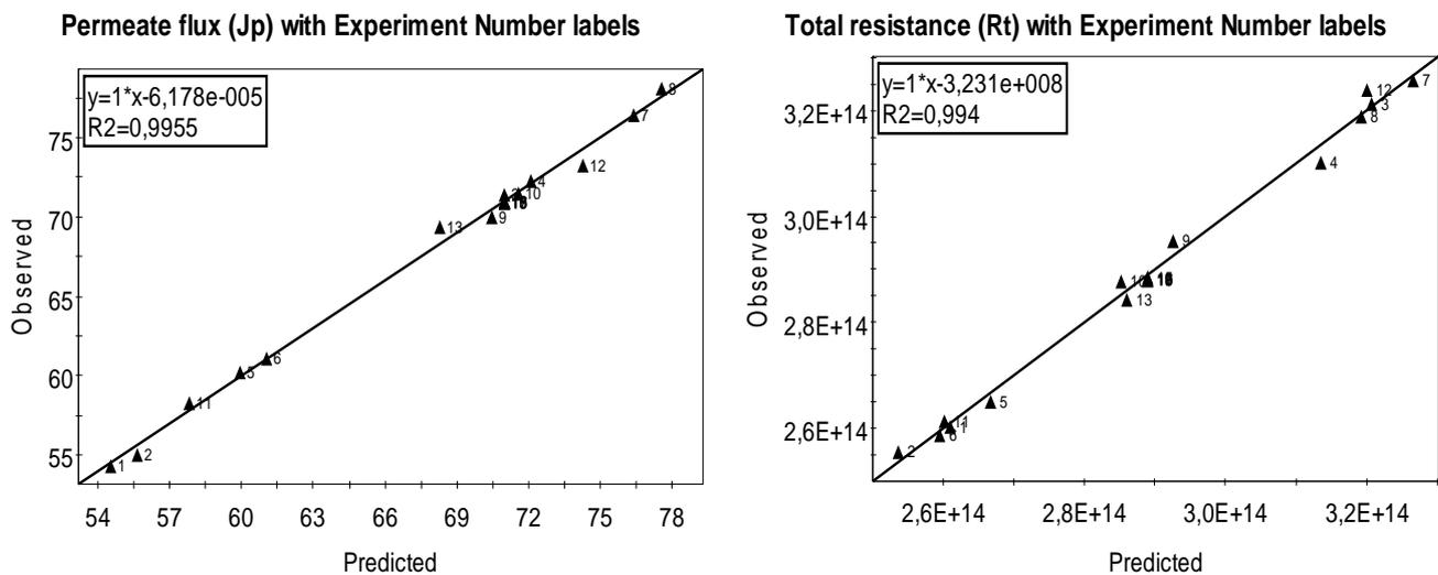
Fig. 2. Observed versus predicted values for permeate flux and total resistance
