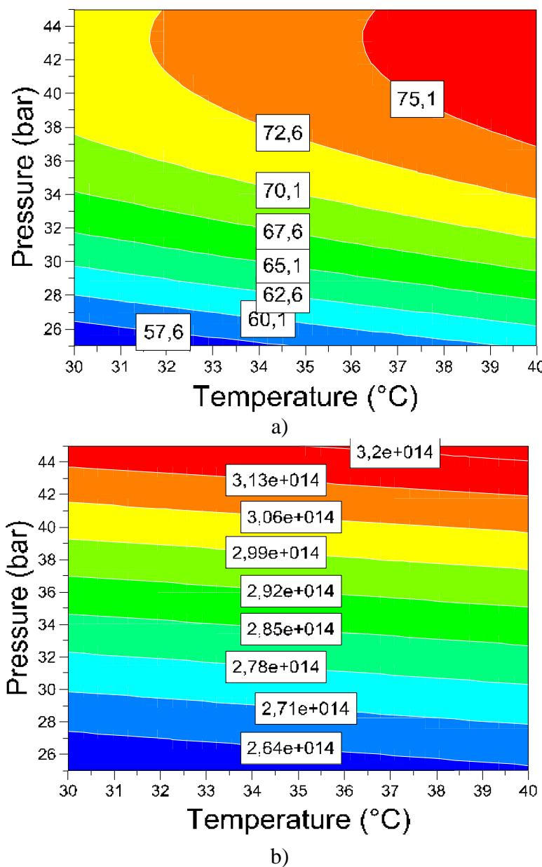
Fig. 3. The combined effect of temperature and pressure on permeate flux (a) and  $R_t$  total resistance (b)
