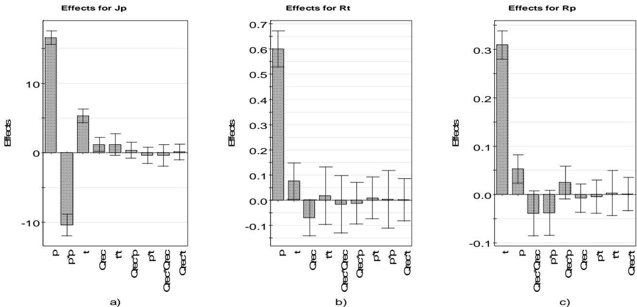
Fig. 1. Effects of factors and interactions on the permeate flux (a), total resistance (b) and polarization layer resistance (c).
