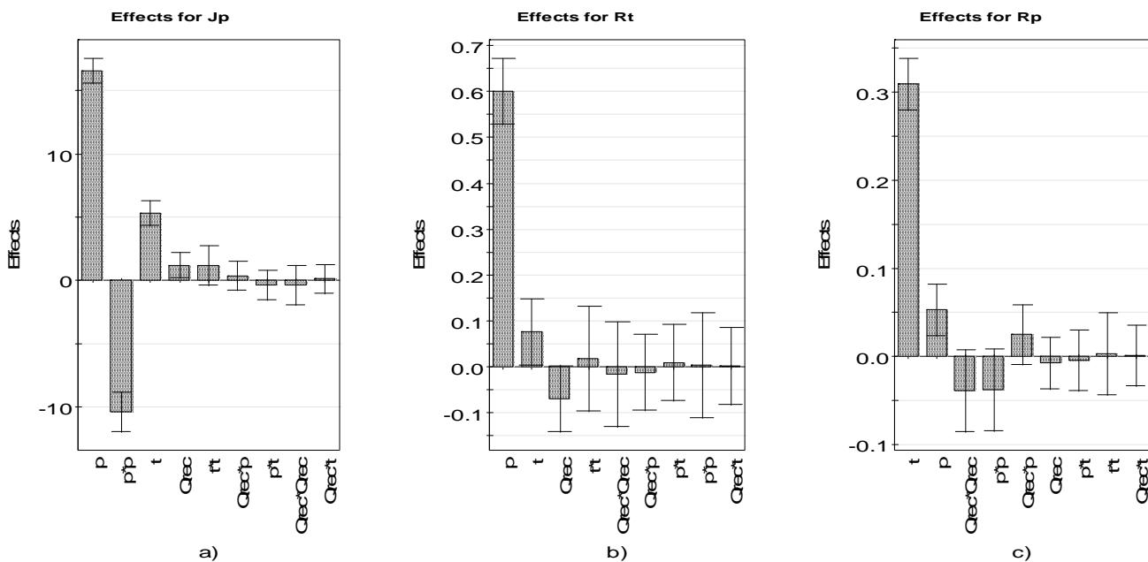
Fig. 1. Effects of factors and interactions on the permeate flux (a), total resistance (b) and polarization layer resistance (c).
