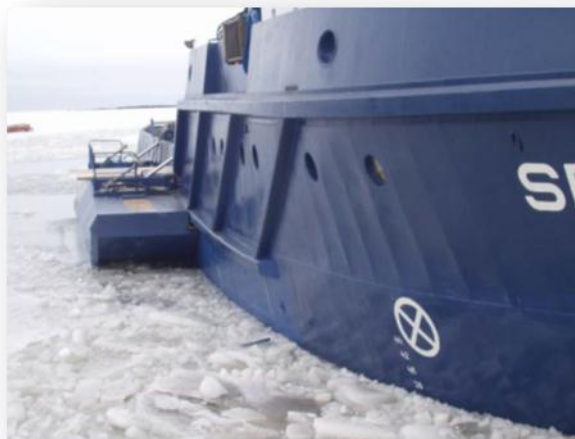
Photo 7. LOIS unit installed on a fair service vessel. Photo by SYKE.
