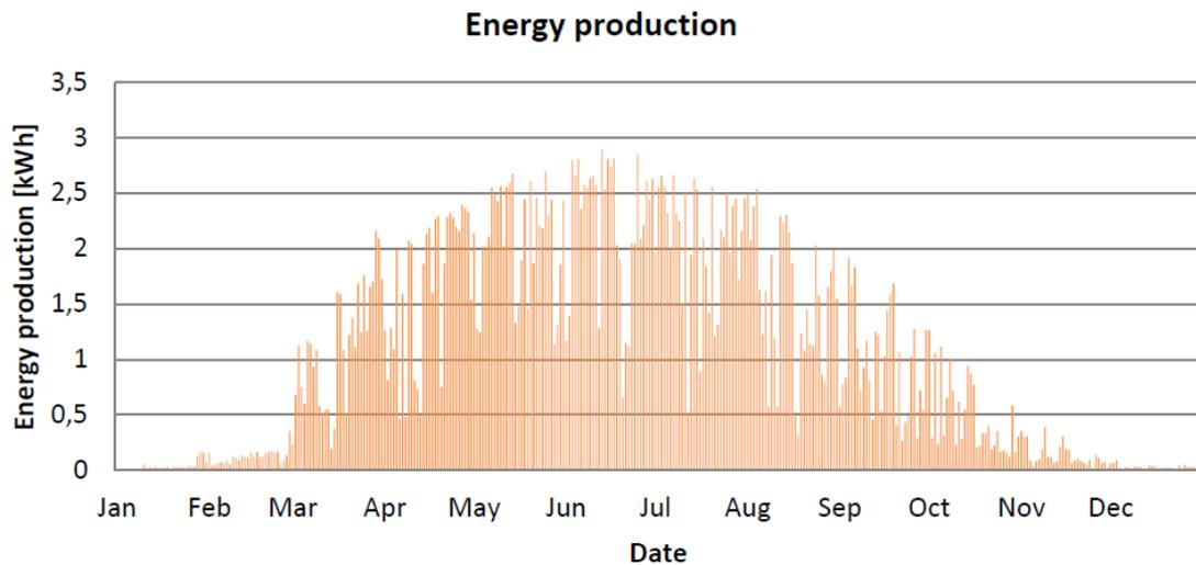
Figure 6. Energy production of PV in Tyrnävä
