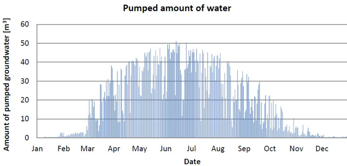
Figure 7. Pumped amount of groundwater in Tyrnävä
